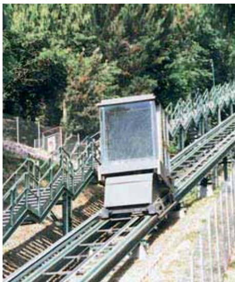
INCLINED LIFT WITH CONSTANT INCLINE Rated load 2250 n° 2 stops in line Constant incline 24° Travel 134 m
