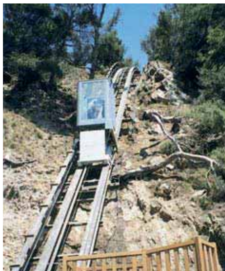
INCLINED LIFT WITH VARIABLE INCLINE Rated load 450 kg n° 2 stops in line Variable incline 20-48° Travel 68 m
