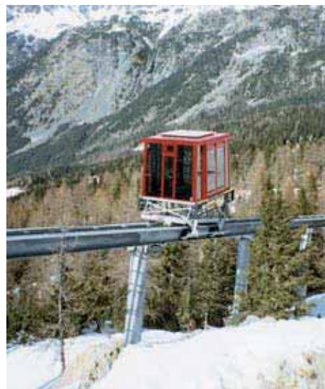
INCLINED LIFT IN PUBLIC SERVICE WITH CONSTANT INCLINE Rated load 3000 kg n° 2 stops in line Constant incline 11° Travel 350 m
