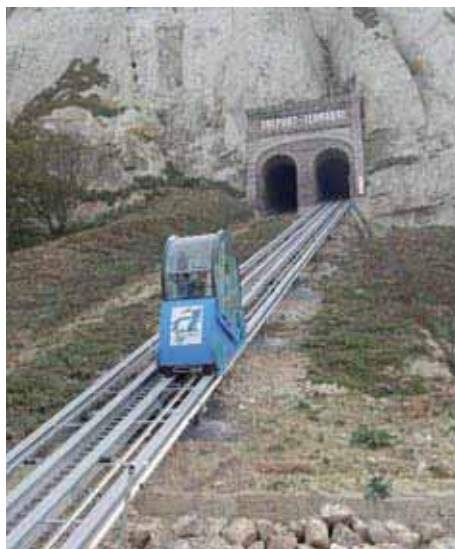
TREPORT - FRANCE Inclined lifts in public service Rated load 1075 kg Constant incline 32° Travel 160 m
